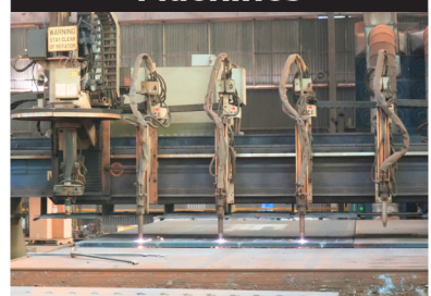
8 Oxy Fuel Cutting Machines
